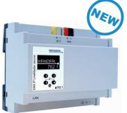
The device combines the central functions of a KNX bus line: Bus power supply with bus choke, KNX IP router and KNX IP interface with low space requirement. Comprehensive diagnostic functions. The KNX IP router in the LineMaster enables the forwarding of telegrams between different lines via a LAN (IP) as a fast backbone. The device also serves as a programming interface between a PC and the KNX bus (e.g. for the ETS®).
