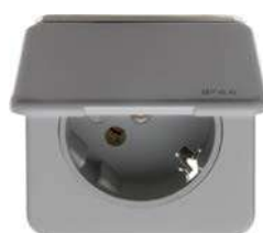
Built-in SCHUKO socket outlet 45° with hinged cover, SNAP IN 1.3 - 2.2 mm, imprint "IP 44"
